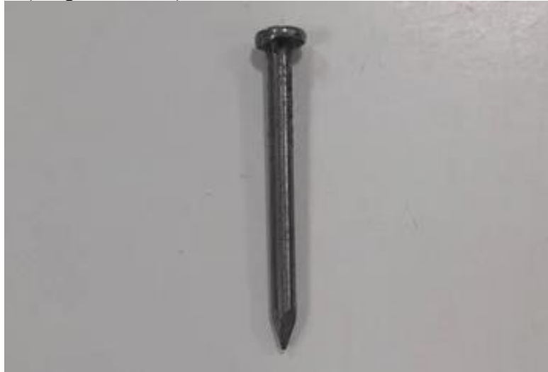
Figure 4: Steel nails (Length: 25.4 mm)
