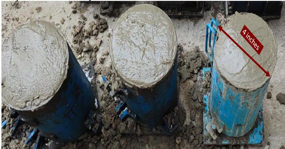
Figure 5: Preparation of concrete cylinders with steel nails
